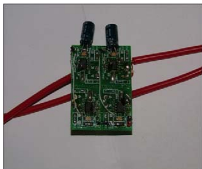
Fig. 10: prototype of Active Bridge
