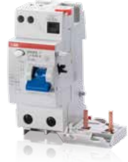
DDA 202 Type F , RCD blocks (to be mounted with S202 MCBs) in two poles with rated current 40 and 63A and sensitivity 30mA for quick and flexible solutions.
