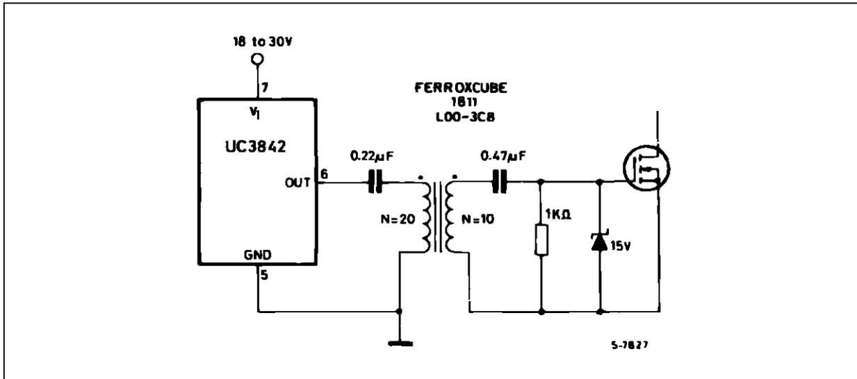
Figure 17 : Bipolar Drive with Negative Turn-off Bias.
