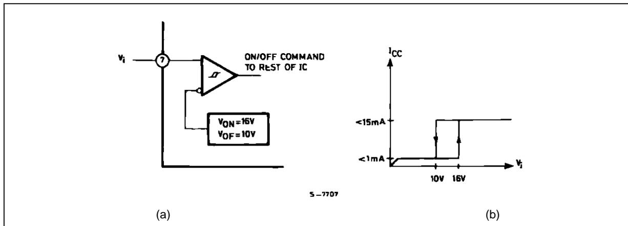
**Figure 6 :** Providing Power to the UC3842.
