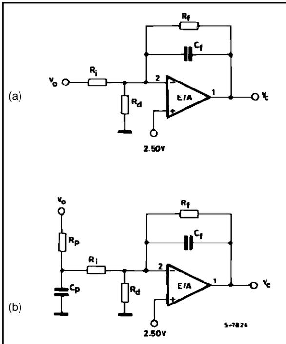
It is therefore desirable to keep the value of  $R_i$  as low as possible.
