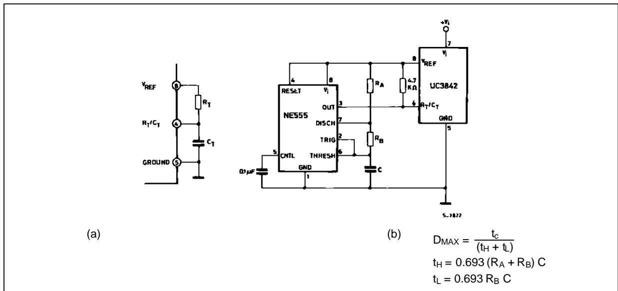
Figure 8 : Synchronization to an External Clock.
