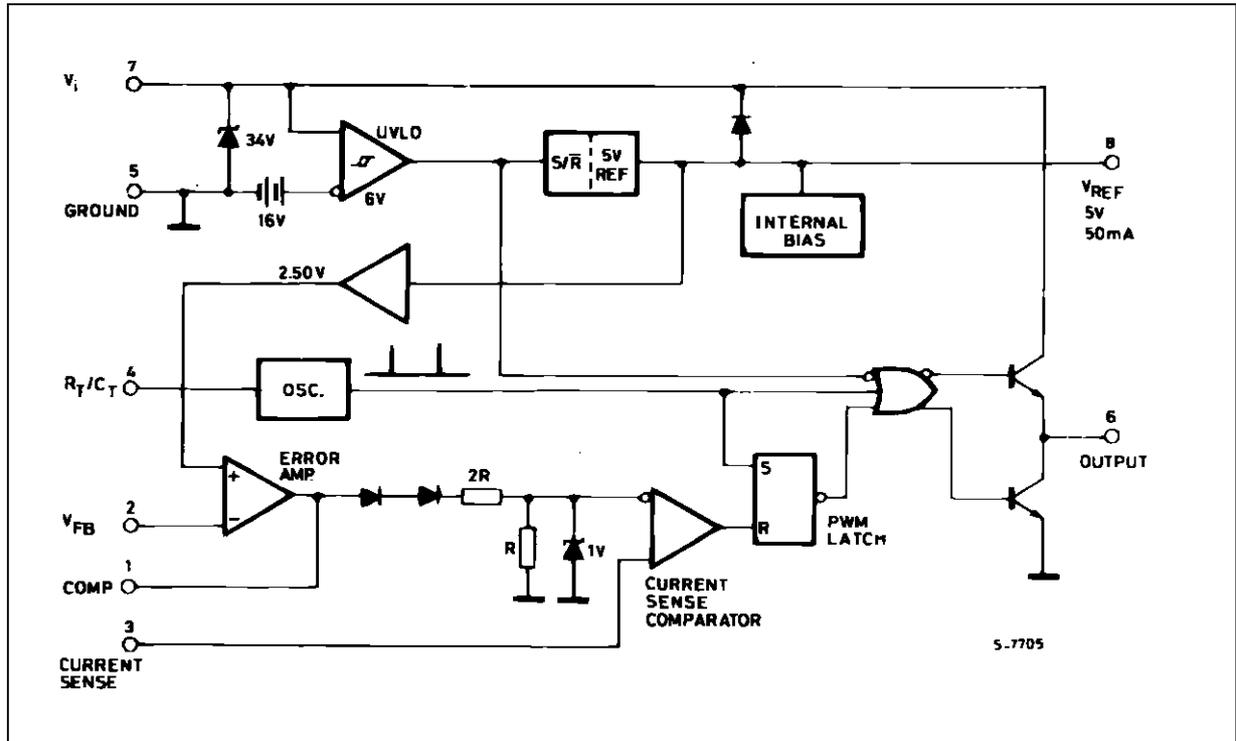
Current limiting is simplified with current-mode control. Pulse-by-pulse limiting is, of course, inherent in the control scheme. Furthermore, an upper limit on the peak current can be established by simply clamping the error voltage. Accurate current limiting allows optimization of magnetic and power semiconductor elements while ensuring reliable supply operation.
