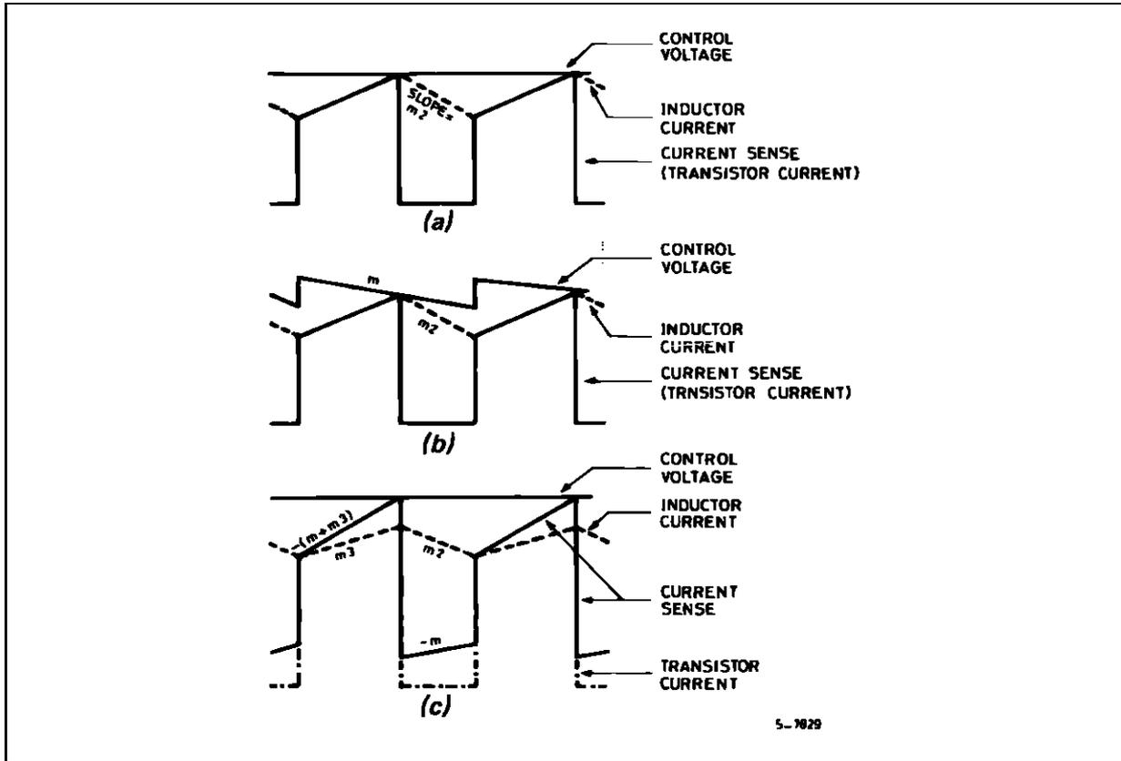
Note that in order for the error amplifier to accurately replicate the ramp,  $Z_F$  must be constant over the frequency range  $f_s$  to at least  $3 f_s$ .
