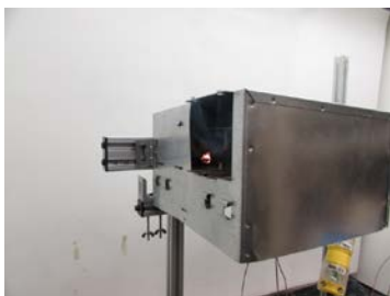
The large flames subside and the winding wrap and/or the winding coating appears to be burning
