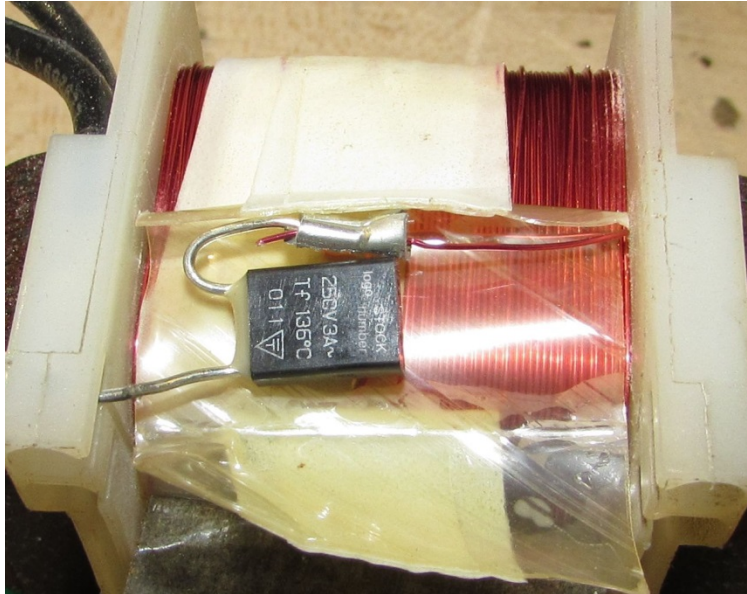
Figure 6. Radial eutectic-type thermal fuse in the sample fans
