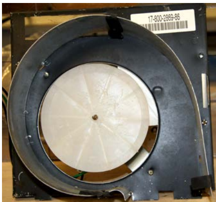
Top of the exhaust fan assembly
