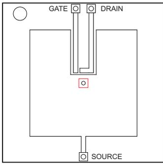
Max  $R_{\theta JA} = 63^{\circ}\text{C/W}$
