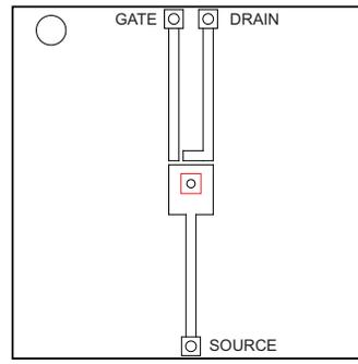
Max  $R_{\theta JA} = 165^{\circ}\text{C/W}$
