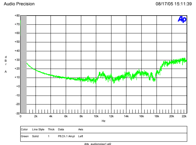
Figure 30 – Audible Noise V_{IN} = 120 VAC; I_{OUT} = 1 A.
