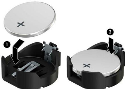
7. **Type 3:** Pull back the clip (1) that is holding the battery in place, and remove the battery (2).
