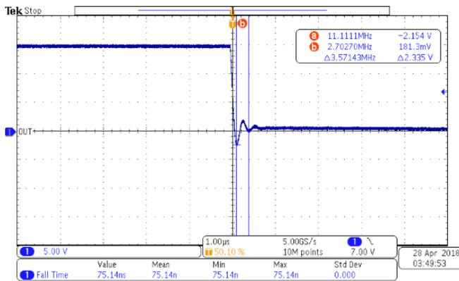
Figure 4. External Gate Resistor  $R_{GATE} = 0\text{-}\Omega$
