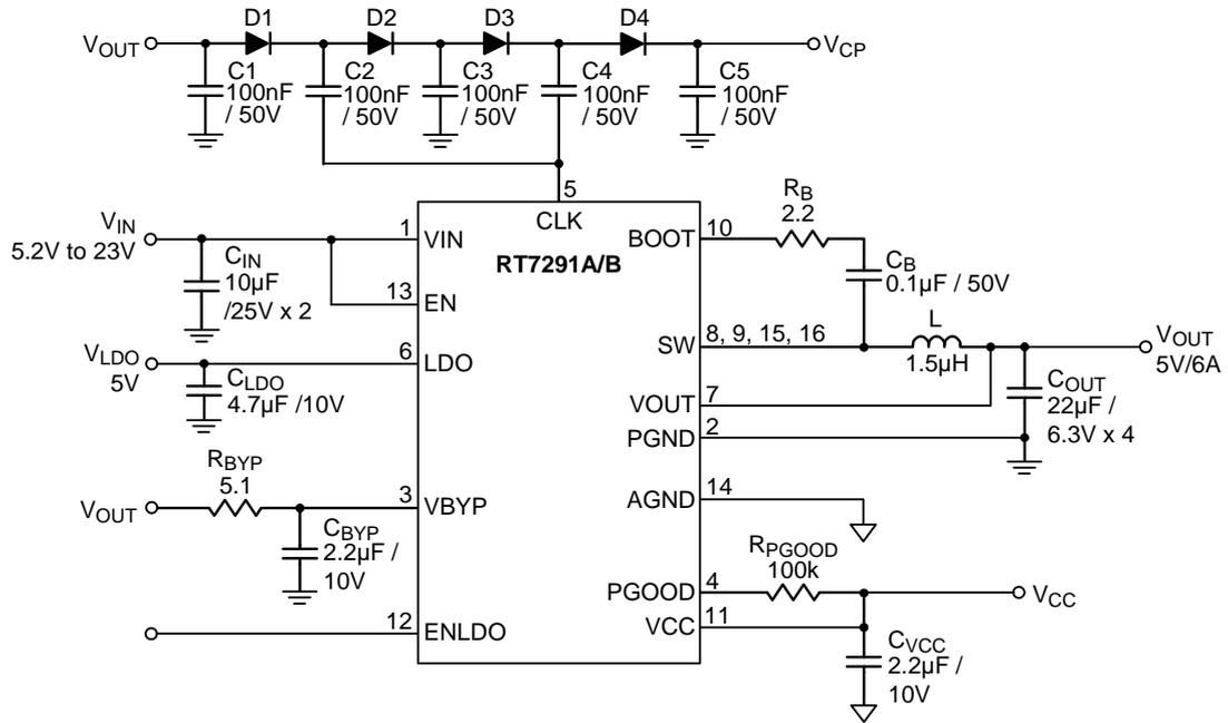
Figure 1. Typical Application Circuit with Pure MLCC Solution
