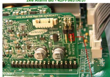
2K6 Alarm Bd - 42PF9631A/37 Place 2 Pin Jumper over BJ8901 (VS ON Int.) pins to troubleshoot PDP without SSB.
