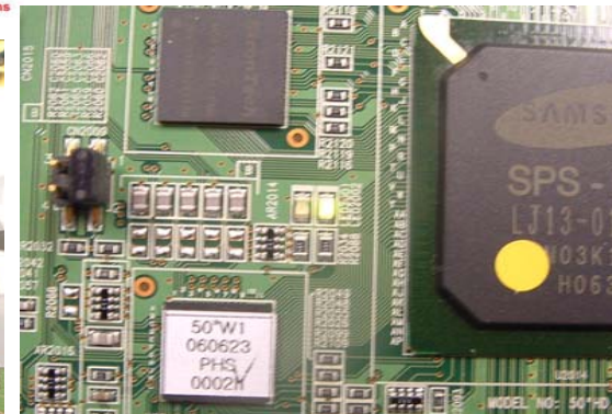
Two LED's - left turns On, then right LED starts blinking and then left LED turns Off Jumper On pins 1 & 2 to left of LED's
