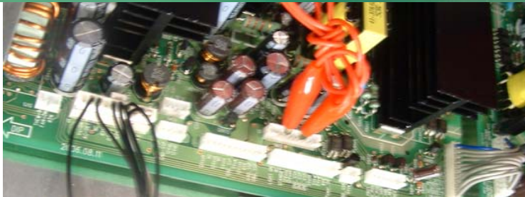
1M03 Pins 4 (GND-SSP) & 7 (STANDBY) - Sub Power Supply
