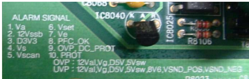
2k6 PSU Alarm signals printed on PSU
