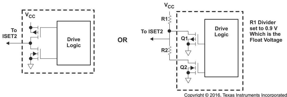
图 9-6. Configurations for Driving the 3-State ISET2 Pin
